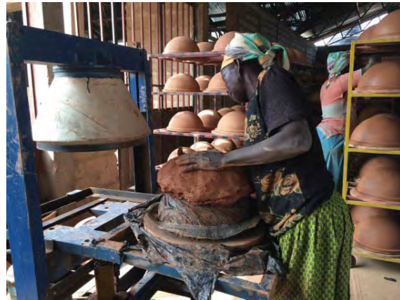
Figure 3-19 Putting the clay/rice husk mixture on the Male Mold
