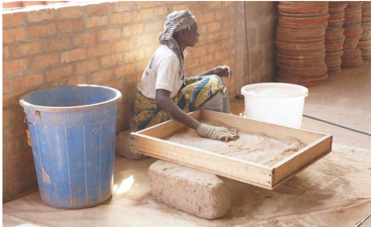
Figure 3-11 Sieving process at PHW factory
