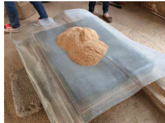
Figure 3-13 Put rice husks on top of mesh screens
