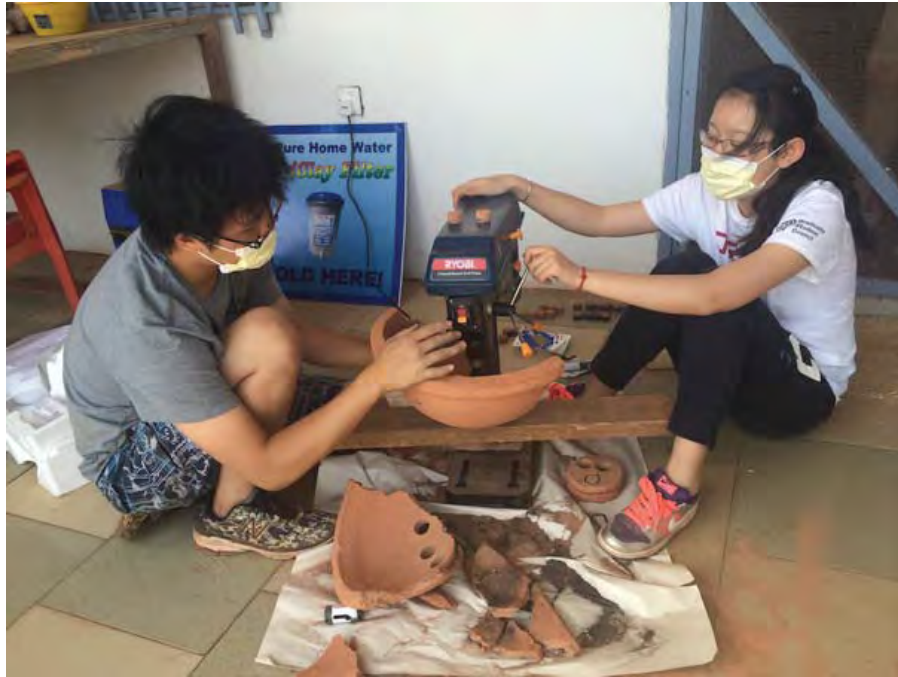
Figure 3-5 The drilling process using a drill press
