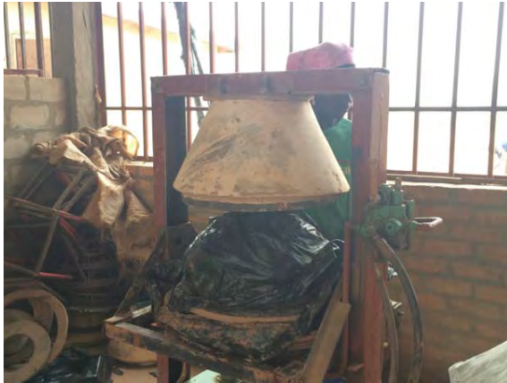
Figure 3-18 The Hydraulic Press showing Male & Female Molds
