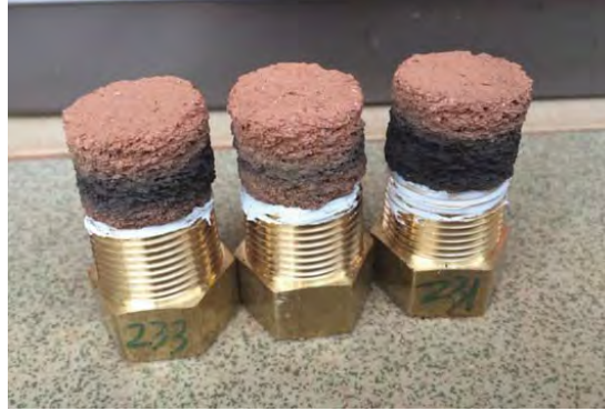
Figure 3-3 Group T F with glue attaches sample ceramic disks to brass fittings but without silicon glue on side faces
