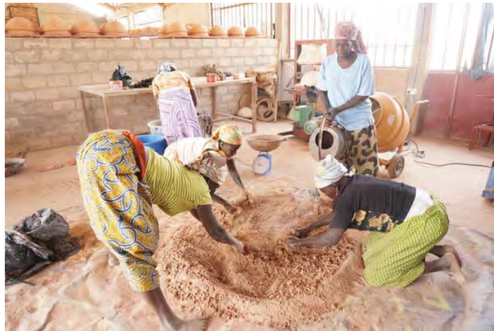
Figure 3-17 Adding water to the mix
